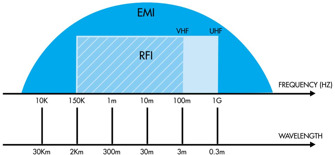
Fig. 1.0 Frequency range for EMI and RFI
